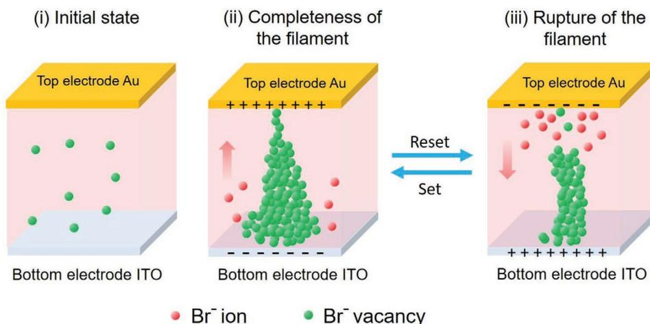
**Figure 4.** Illustration of the conductive filament formation and resistive switching mechanism of the as-prepared memory device.
