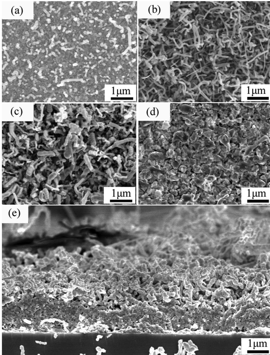
**Fig. 2.** SEM images of GaN samples at different temperatures: (a) 850 °C, (b) 900 °C, (c) 950 °C, (d) 1000 °C and (e) the cross-section image of the Fig. 2(b).
