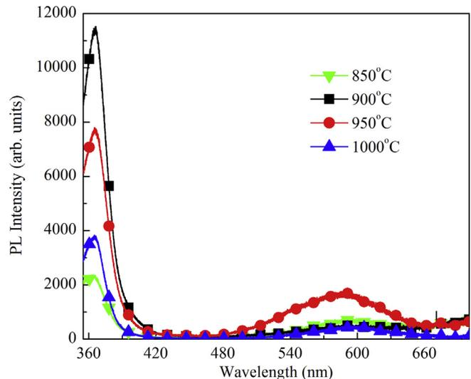
**Fig. 3.** PL spectra of GaN samples at different temperatures.
