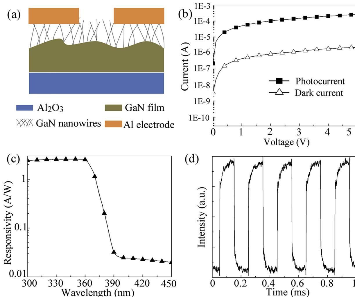
Fig. 4. (a) A diagram of the UV detector based on GaN nanowire-film hybrid films, (b) I-V characteristics, (c) Spectral responsivity, and (d) Transient response.
