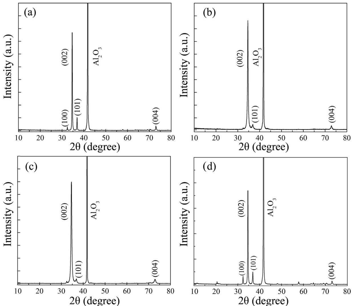
Fig. 1. XRD patterns of as-grown samples at different temperatures: (a) 850 °C, (b) 900 °C, (c) 950 °C and (d) 1000 °C.
